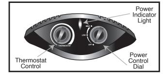
**POWER CONTROL DIAL:** This heater has two heat settings: High and Low. Use the higher setting (1500W) to raise the room temperature quickly. When the desired temperature is reached use the Low setting. It is usually sufficient to maintain a comfortable temperature.
